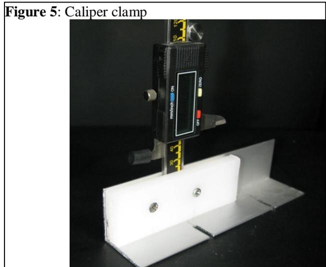
**Figure 5:** Caliper clamp
