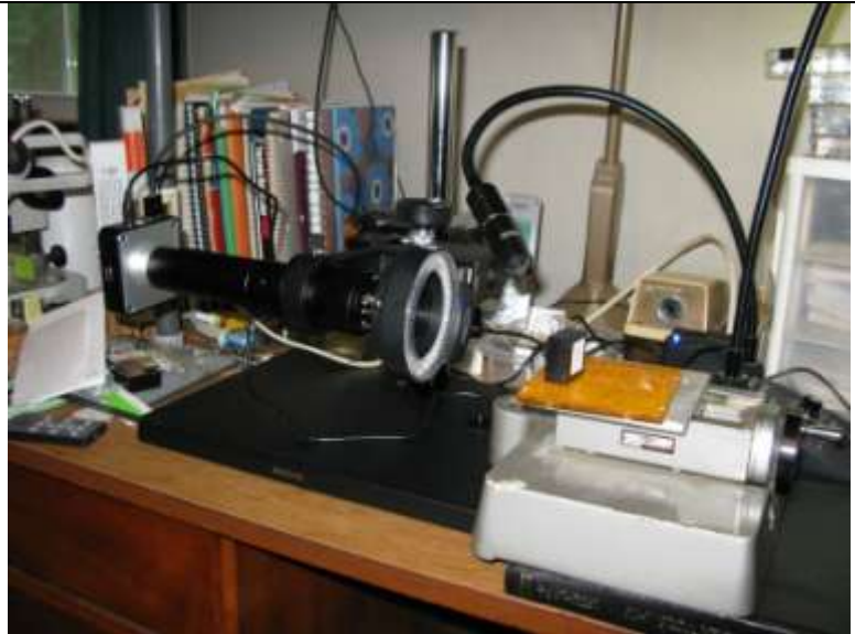
Figure 6 : Hayear camera set horizontally to work with my ultra fine pitch single axis translation table.
