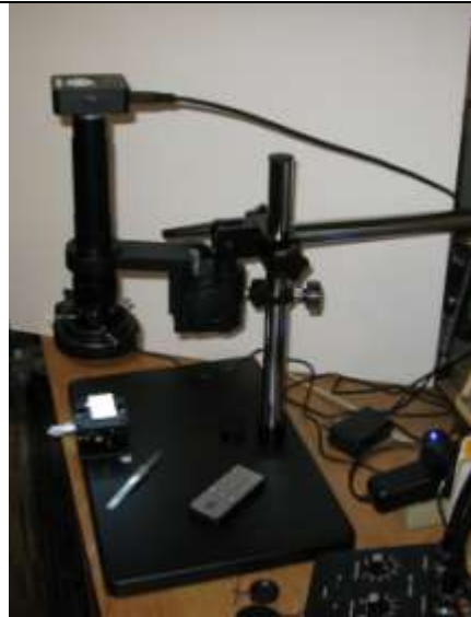
Figure 5 , Hayear camera with micrometer vertical stage for image stacking.
