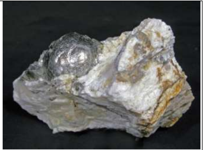
Figure 4: Muscovite – ball mica. 7 cm specimen with 2.3 cm mica ball. T. Mortimer specimen & photo
