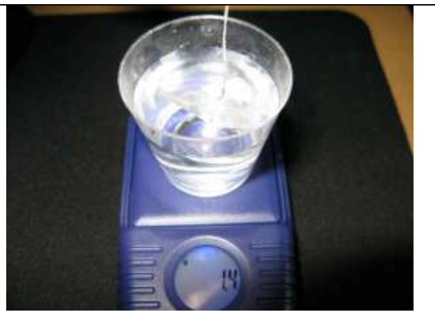
Specimen suspended in water with dental floss.
