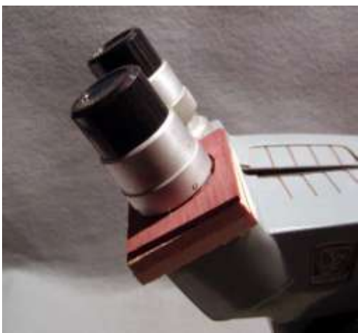
Figure 5: Basswood adapter "stop" on microscope
