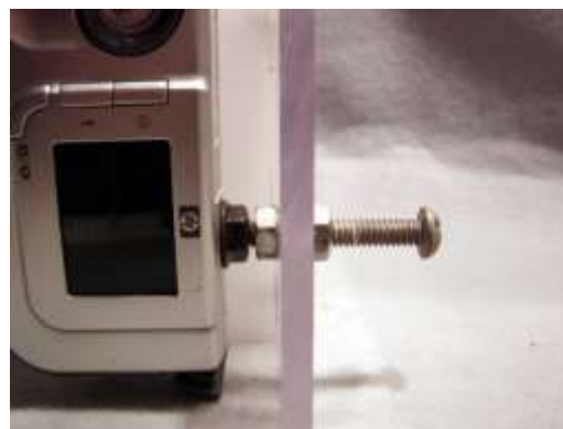
Figure 6: Camera mounting bolt with "y" position adjustment nuts.
