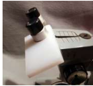
Figure 4: Nylon press-fit microscope attachment piece on American Optical microscope.
