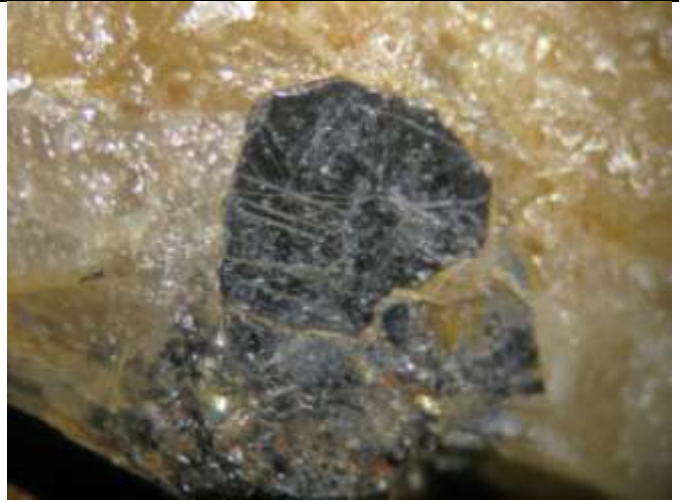
Ilmenite – Visual identification 4 mm ilmenite crystal in quartz. Rutile and clinocllore are also present on this TN sized specimen. This specimen came from the "Green Balloon Prospect" area.
