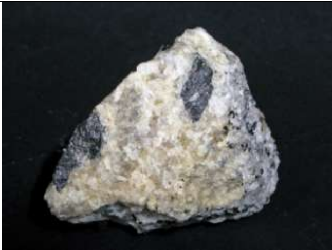
Magnetite in quartz Magnetite identification by strong magnetic attraction. Magnetite has not appeared on previous Richmond Soapstone Quarry species lists.
